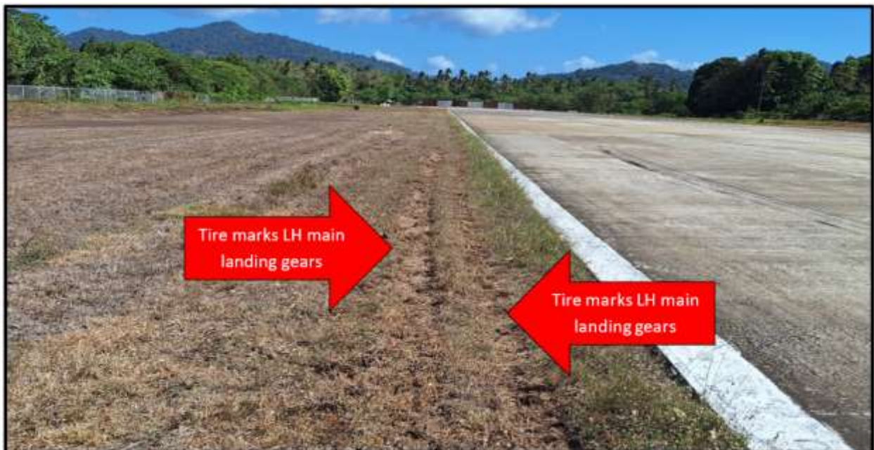
Figure 5 – Off runway tire marks.
