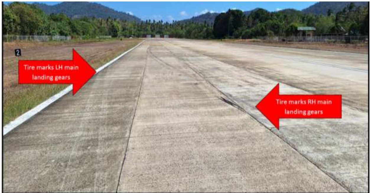
Figure 4 – Tire marks indicating the aircraft LH main landing gears exited the runway and evidence of hard braking actions on the RH main landing gear.
