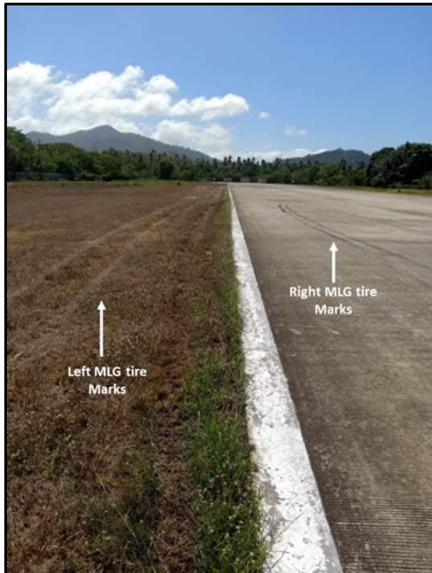
Figure 13 – Aircraft tire marks on the incident site.
