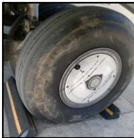
Figure 16 – MLG tires that encountered a runway excursion
