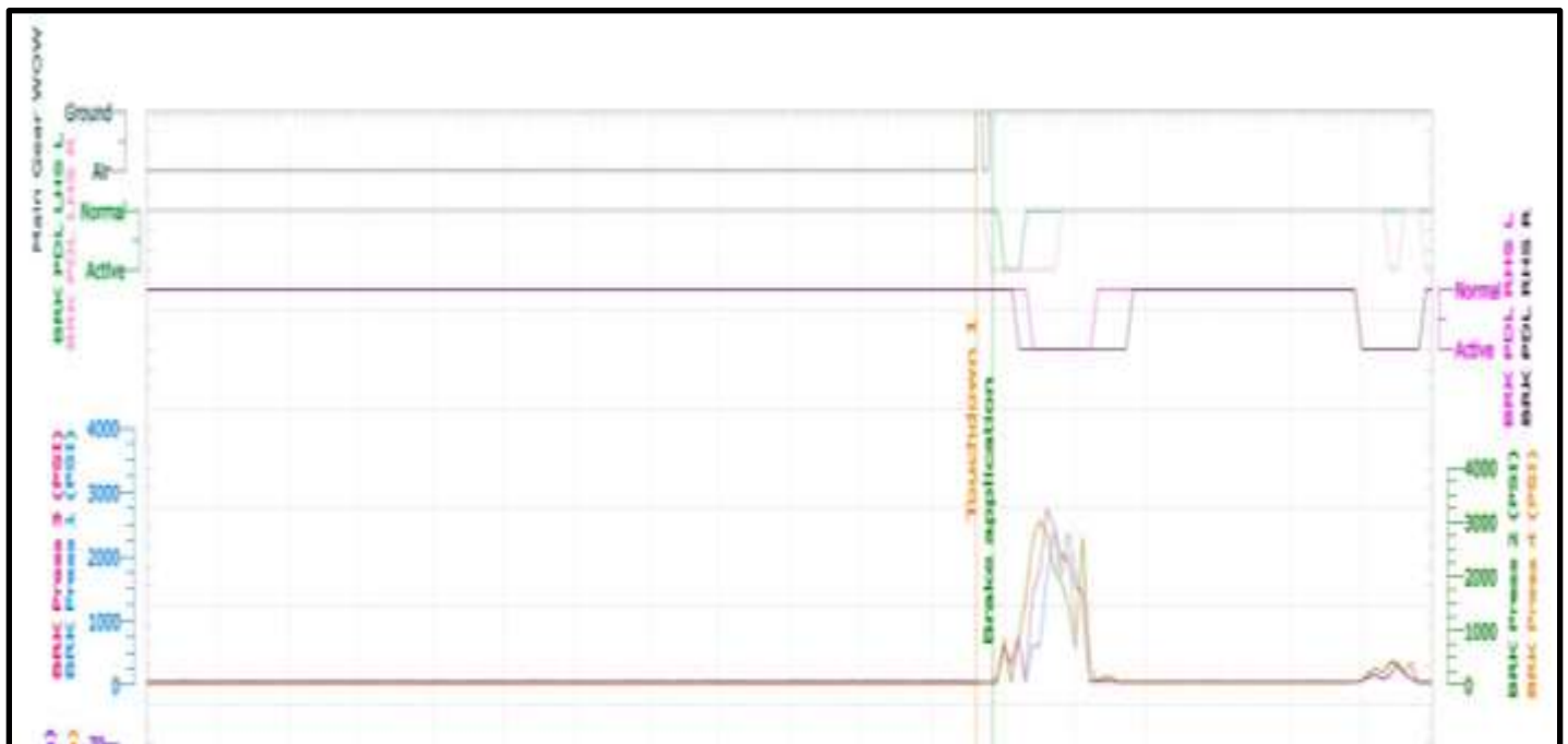
Figure 10 – Braking actions by the flight crew during the landing roll.
