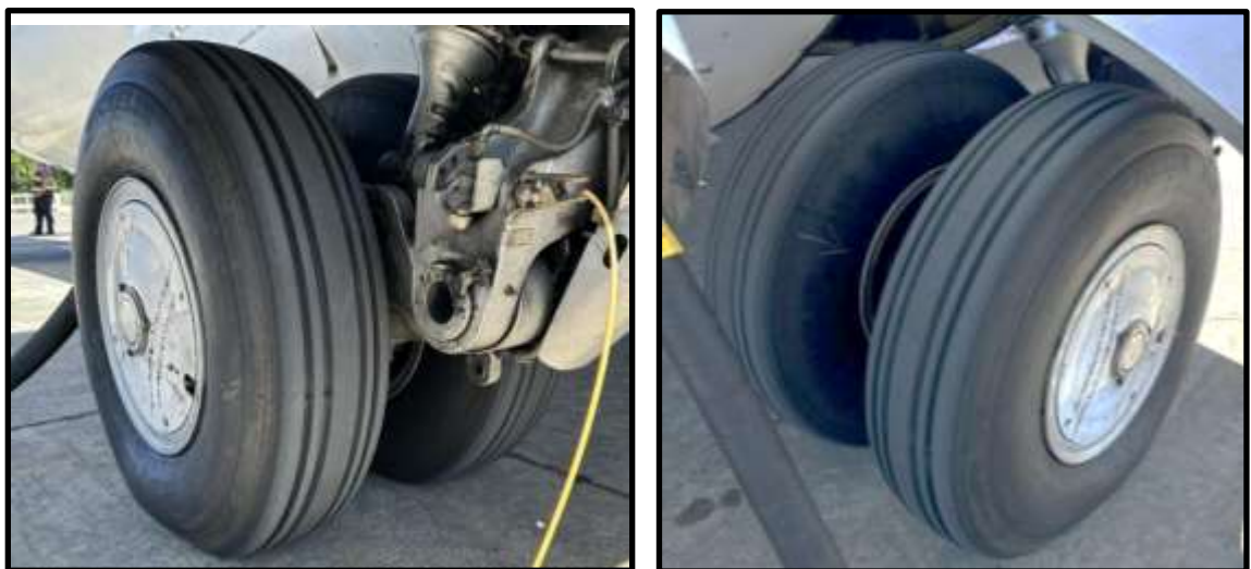
Figure 15 – RH MLG tires after flight ATX-126, which was the 3 rd flight following the incident.
