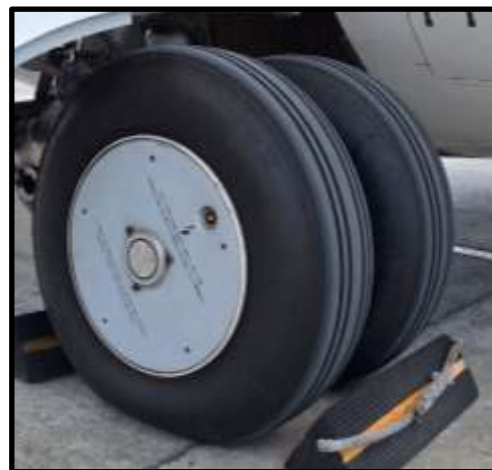
Figure 17 – MLG tires that did not encounter a runway excursion
