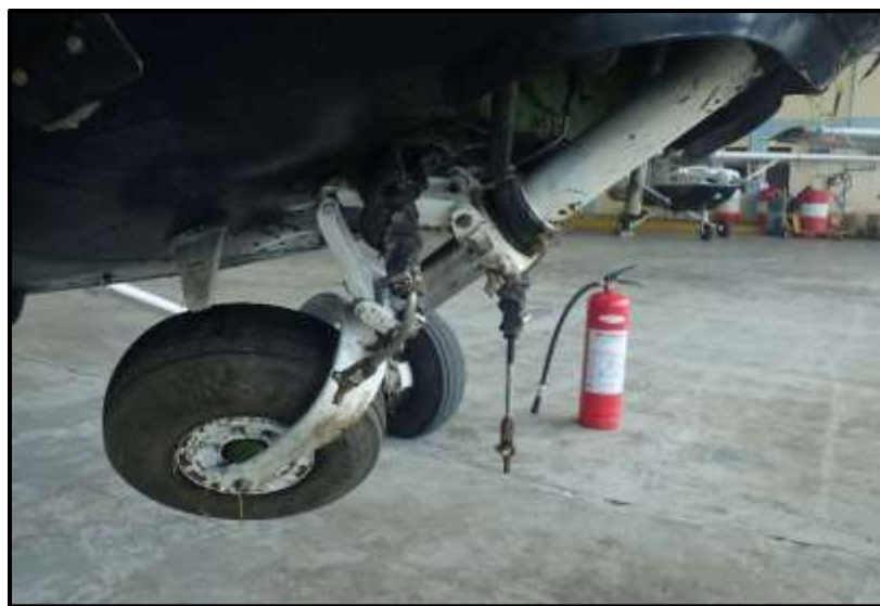
Figure 5 - The damaged NLG left steering tube.
