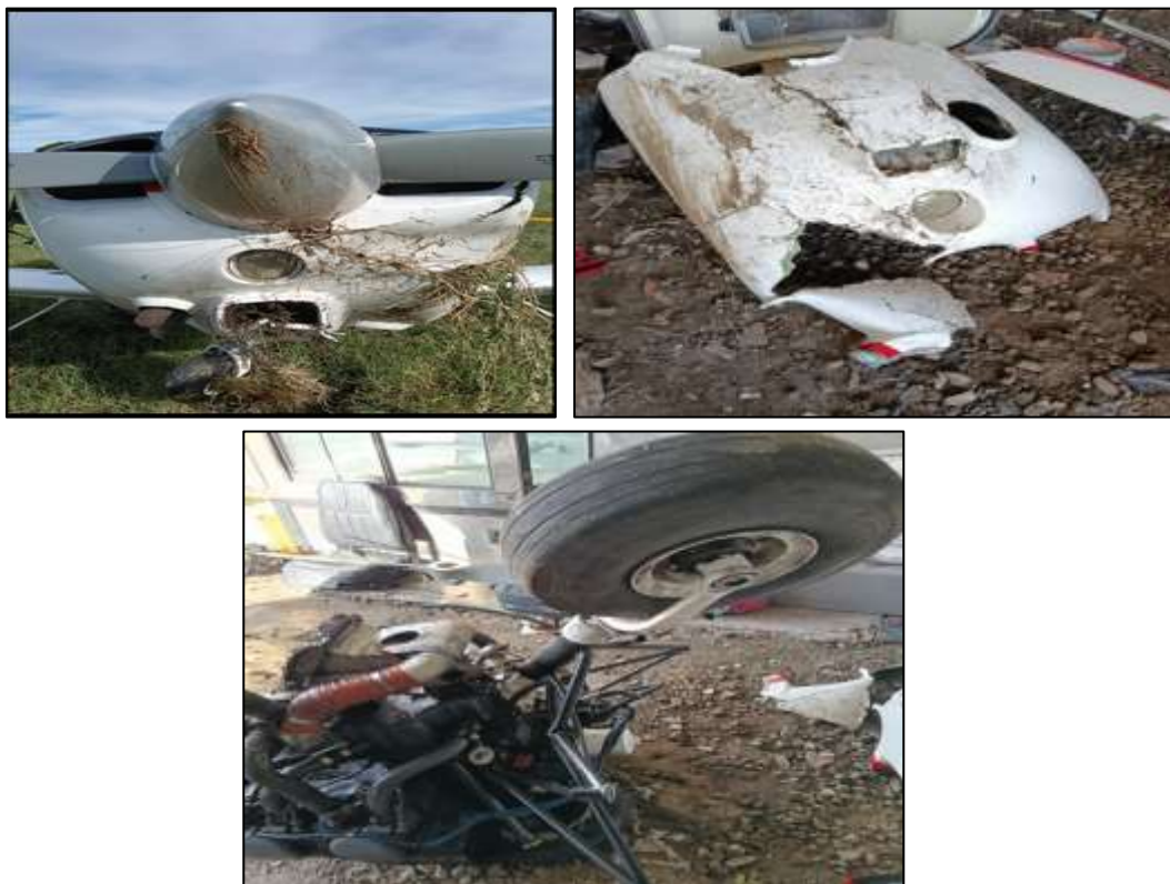
Figure 2 - Damaged Nose Landing Gear (NLG), engine cowlings and engine support.
