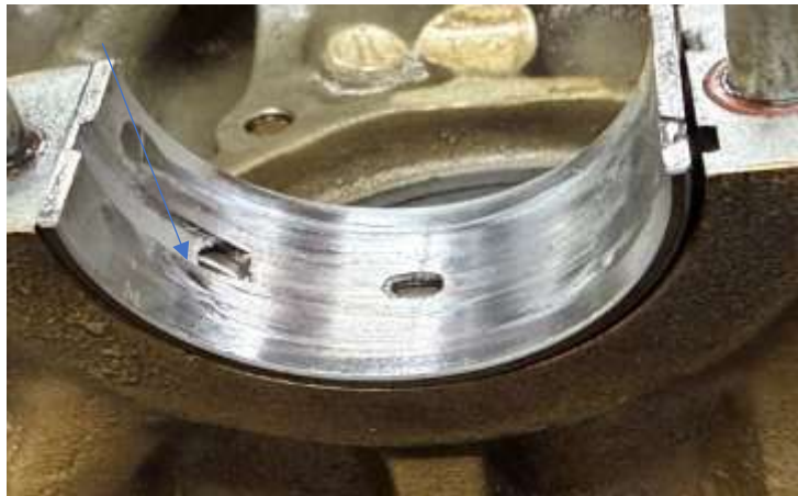
Figure 7 - The Crankcase bearing No.3 holder with scratches.
