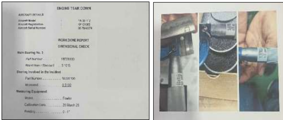
Figure 9 - Dimensions of bearing #3 not within normal dimensions.
