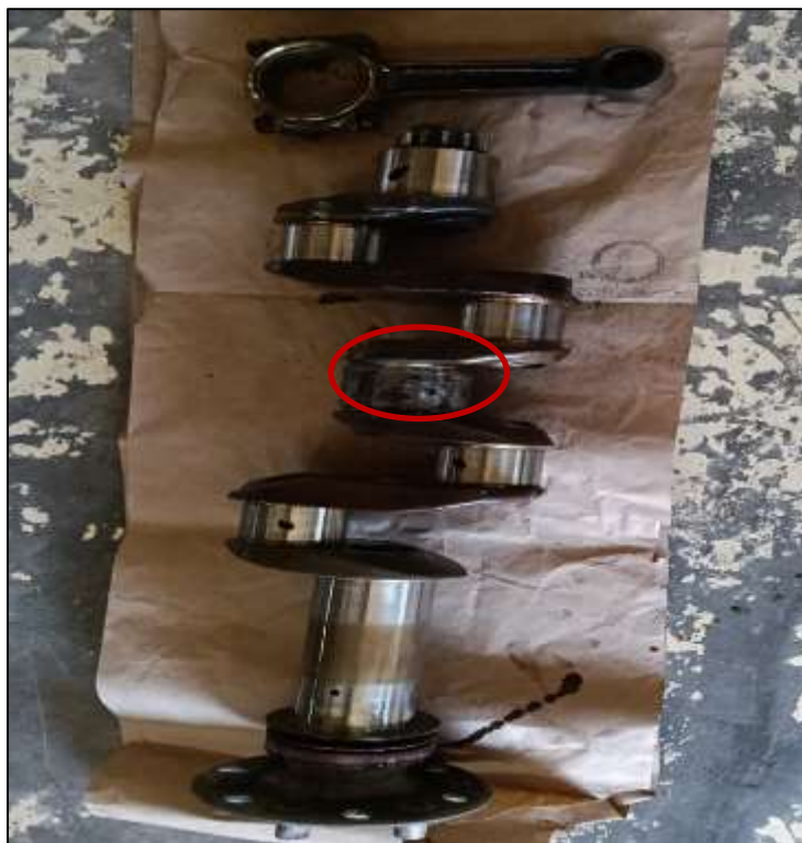
Figure 8 - Showing the #3 bearing still attached to crankshaft.
