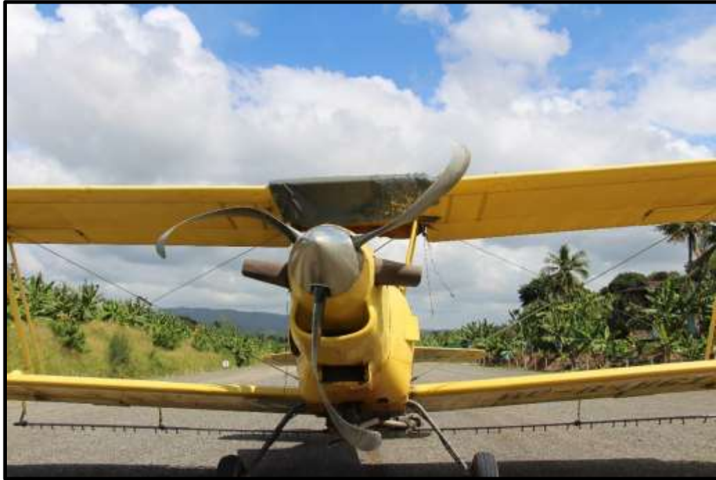
Figure 2: Propeller blades bent at mid span
