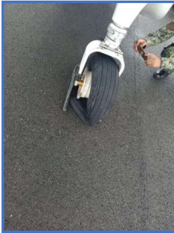
Figure 3: Deflated nose gear strut and tire
