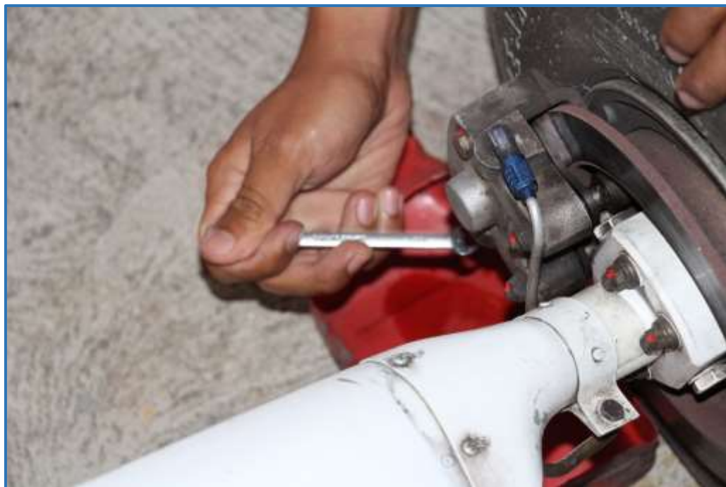
Figure 2: RH brake hydraulic bleeding
