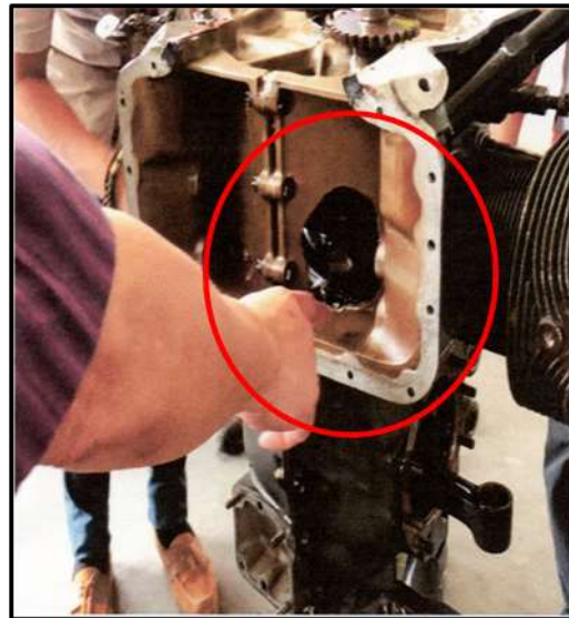
Figure 7. The hole in the crankcase
