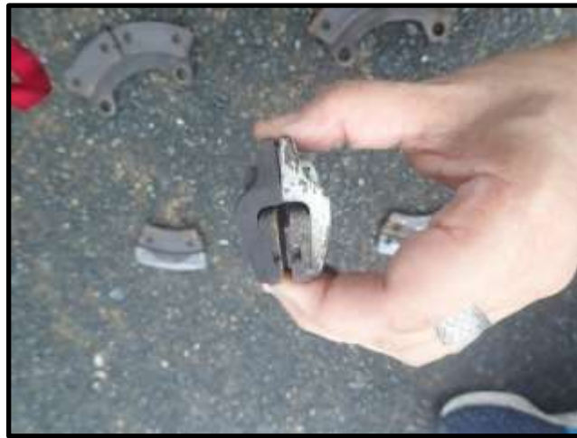
Figure 2. The aircraft left side main landing gear brake pad is thinner than the right side.
