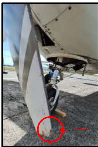
Figures 1 and 2 – Damage (nick) noted on the aircraft propeller.
