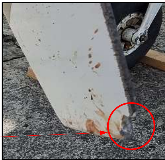
Figures 1 and 2 – Damage (nick) noted on the aircraft propeller.
