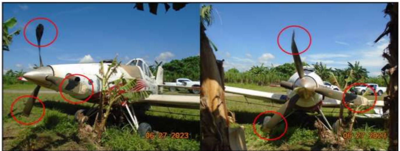
Figure 1 – Bended propeller due to propeller strike.
