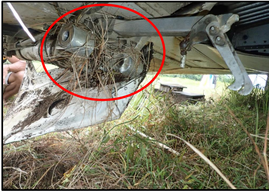
Figure 6. Missing RMLG Shaft Pin.
