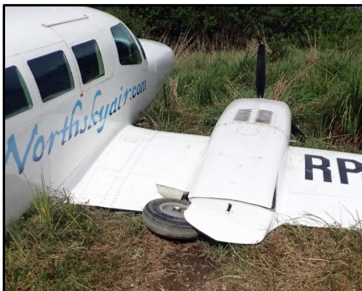
Figure 3. The RMLG did not break away from the aircraft upon landing.
