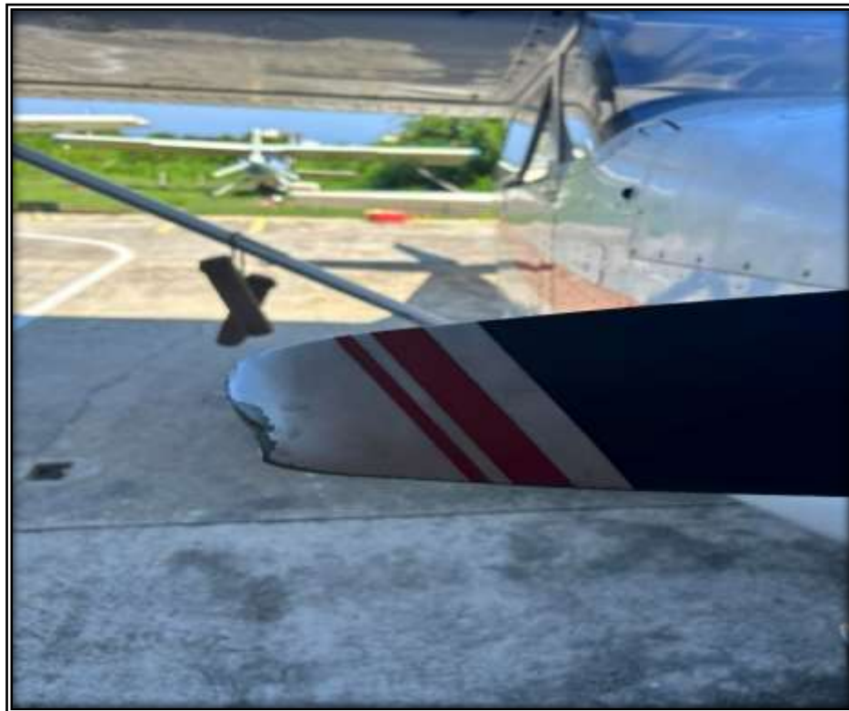
Figure 2: Dent on the propeller blade tip
