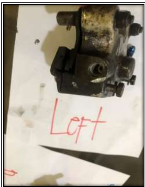
Figure 6 and 7- Dent on part of the aircraft's left main landing gear assembly
