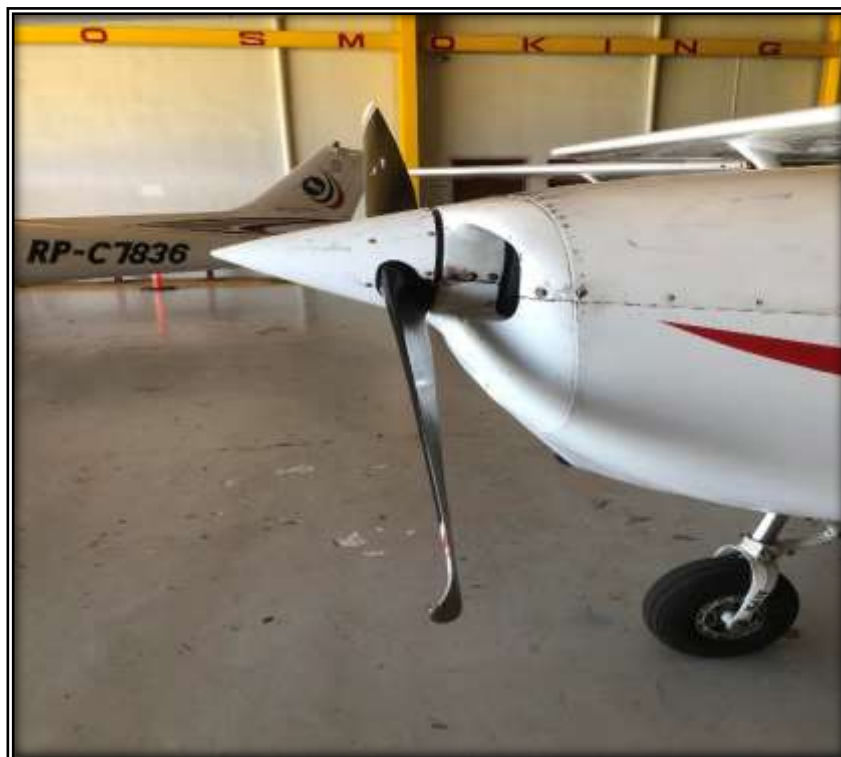
Figure 1. The aircraft bent propeller blade.
