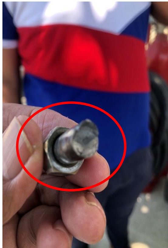
Figure 3 and 4 – Broken Left Main Landing Gear Internal Hex Head Bolt
