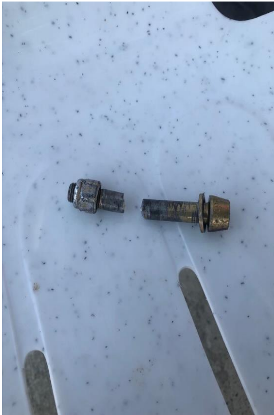
Figure 3 and 4 – Broken Left Main Landing Gear Internal Hex Head Bolt
