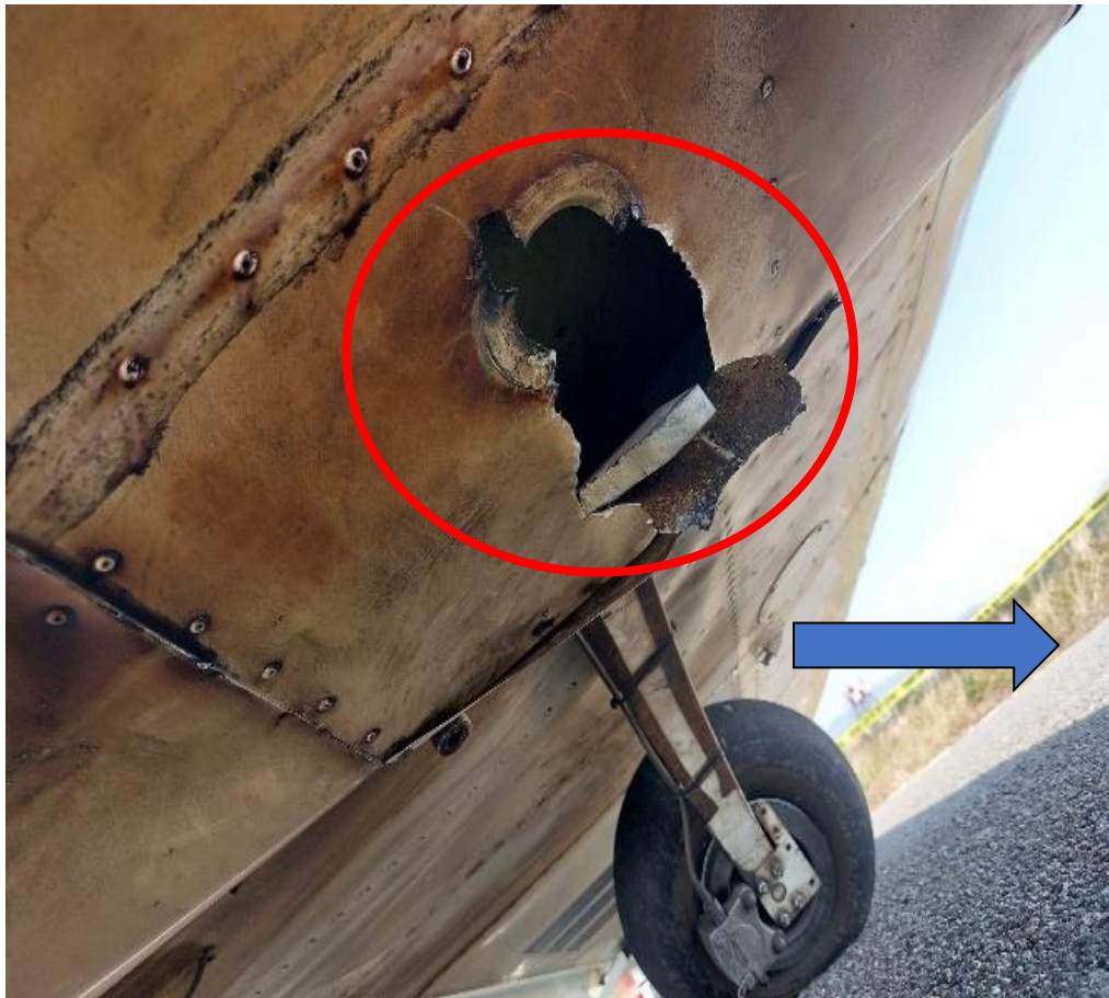
Figure 2 – Left Main Landing Gear leaf spring partially disconnected
