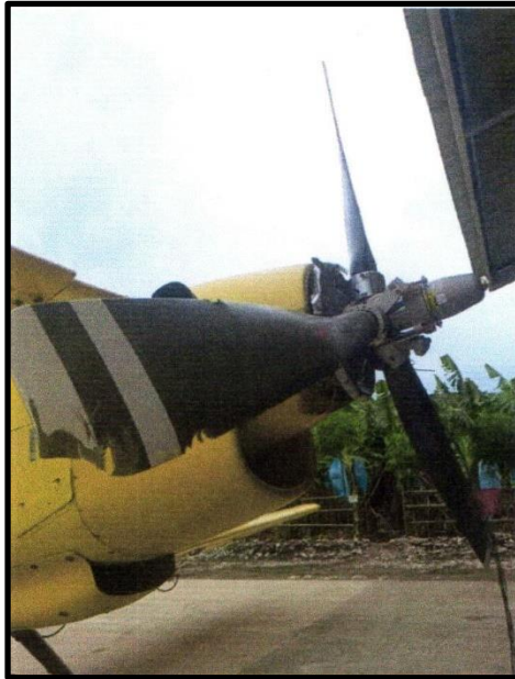
Figure 1. The aircraft with damaged propellers.
