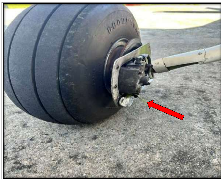
Figure 4: The aircraft's left main landing gear with grasses still stuck at the wheel.
