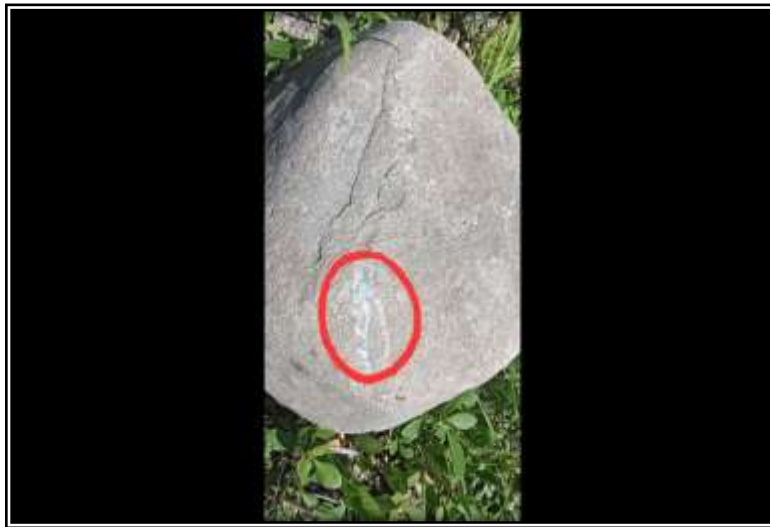
Figure 3: The boulder rock that the aircraft propeller blade hit.
