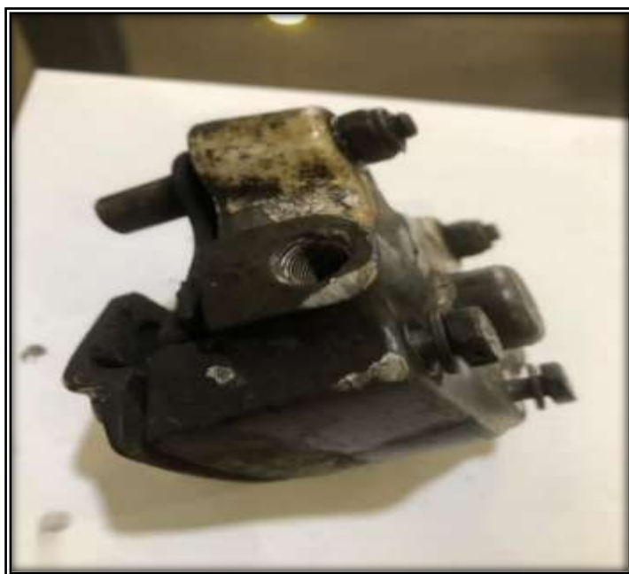
Figure 6 and 7- Dent on part of the aircraft's left main landing gear assembly
