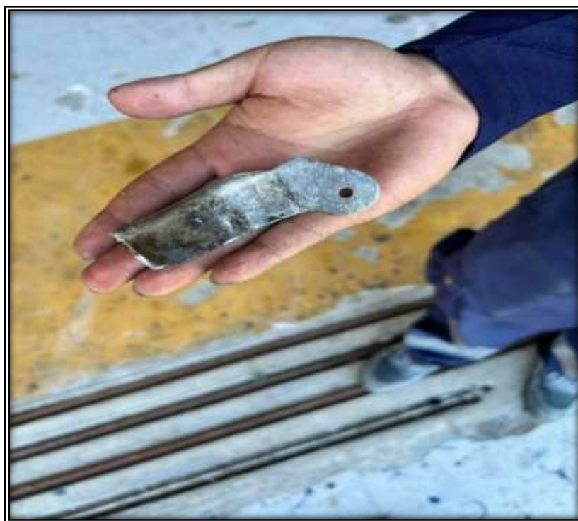
Figure5: Broken part of the aircraft's left main landing gear assembly.
