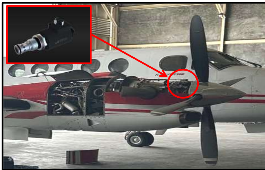
Figure 6. Right-Hand Propeller Auto-feather Low-Pressure switch
