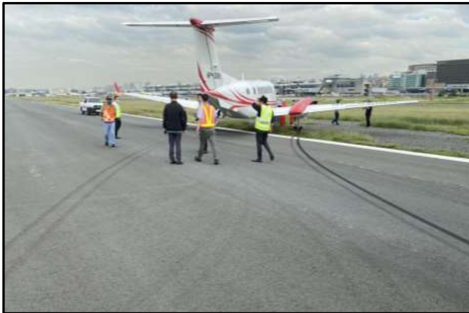
Figure 2 – The aircraft's visible skid marks going out of the runway.
