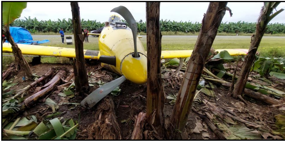
Figure 2: All propeller blades were bent.
