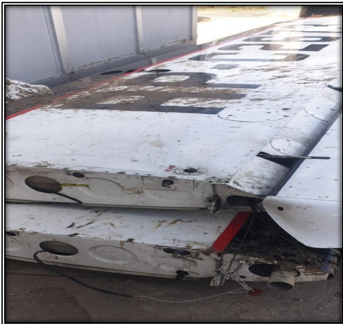
Figure 4 - Aircraft's left and right wing after being removed from the fuselage.
