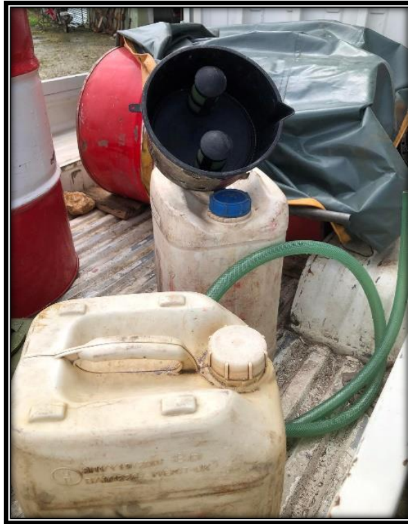
Figure 5 Plastic containers and plastic funnel used for refueling aircrafts
