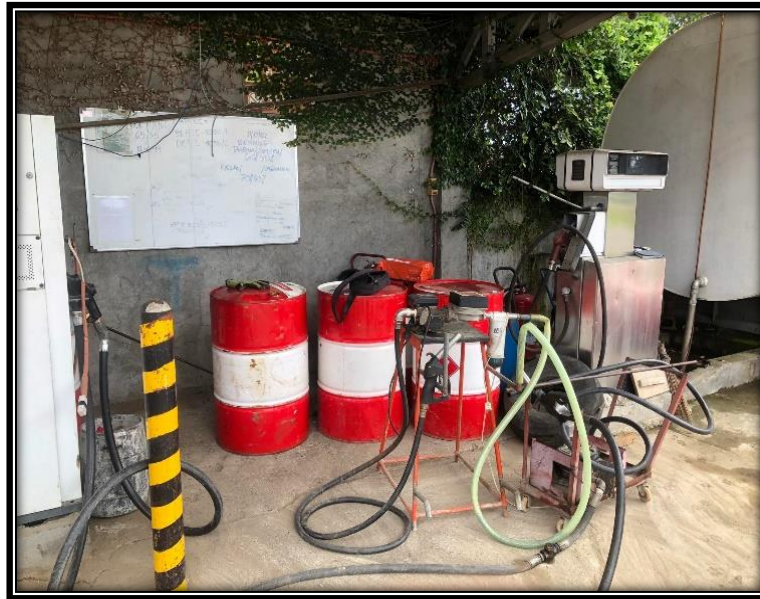
Figure 4 Recycled drums used for multi transfer fueling cycle
