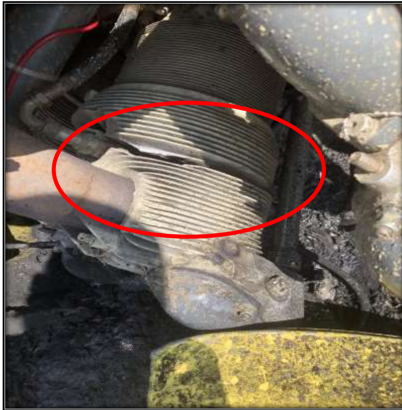
Figure 2 - Crack seen at Cylinder Number 3.
