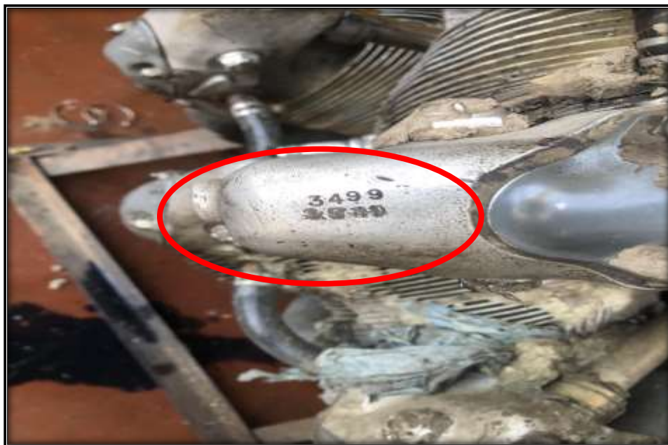
Figure 7 - Cylinder Nos. 5 with markings 3499 stamp.
