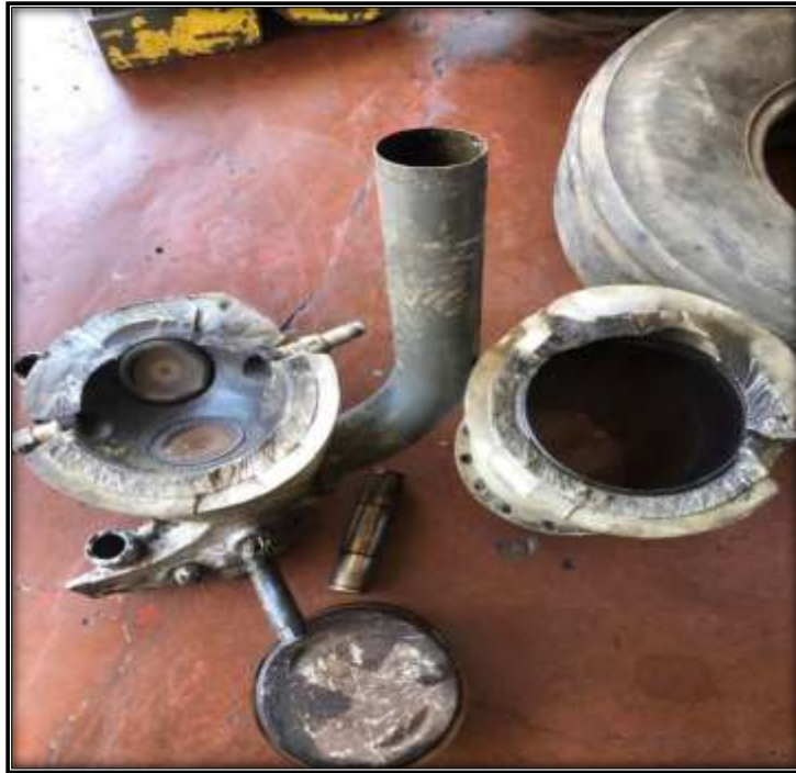
Figure 3 - Separation of the cylinder head from the barrel.
