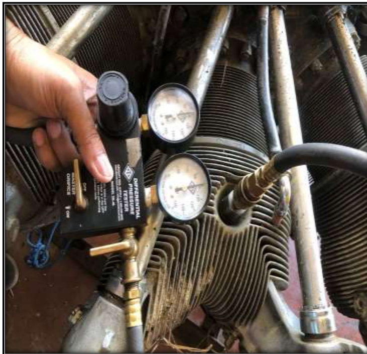
Figure 6 - Cylinder Compression Test
