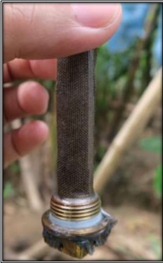
Figure 8 – Carburetor filter upon retrieval.
