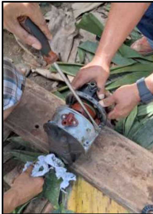
Figure 12 – SPASS personnel checking one of the engine's magnetos.
