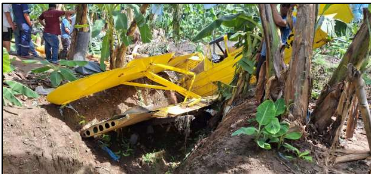
Figure 1 – Aircraft wings were damaged after making contact with the ground.
