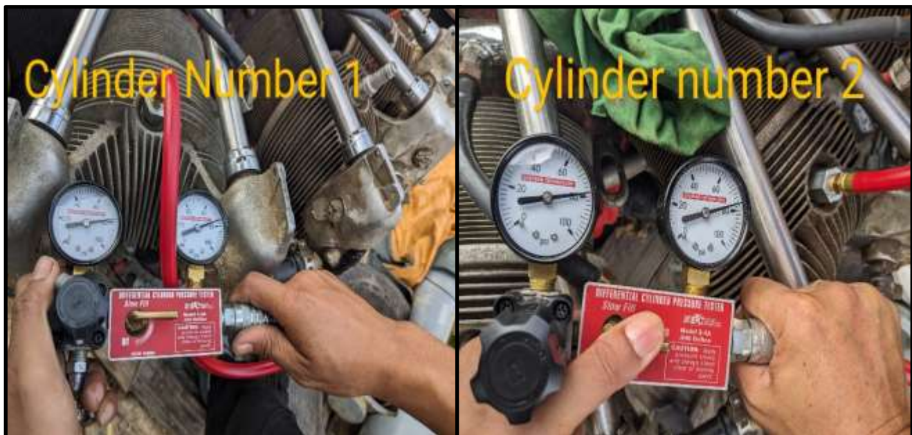
Figure 14 – Some compression checks performed on the engine's cylinders.
