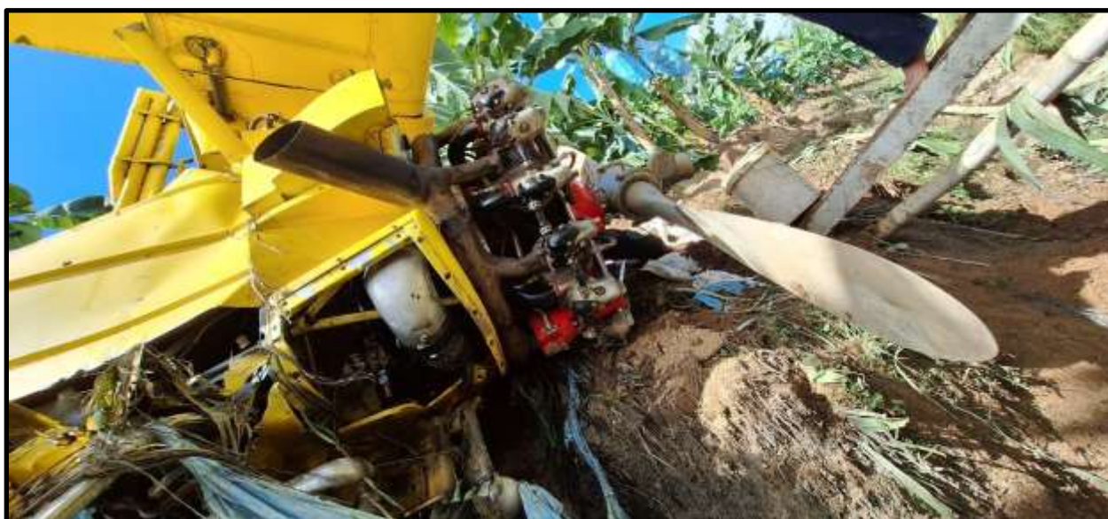
Figure 2 – Damage on the aircraft's lower fuselage and engine.
