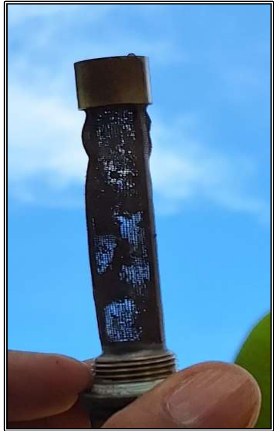
Figure 9 – Carburetor filter after being shaken off.
