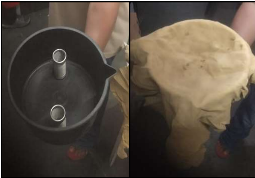
Figure 11 – Funnel and chamois used during refueling.
