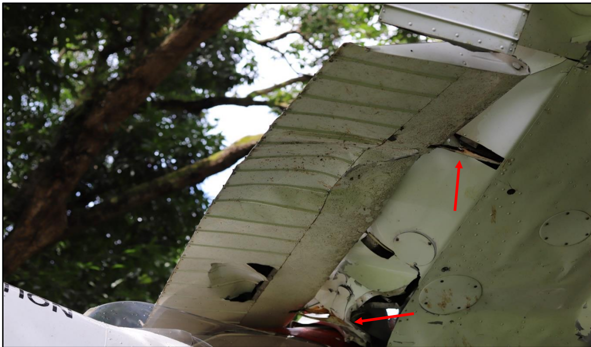
Figure 4: RH flaps in full flaps configuration after impact to a tree
