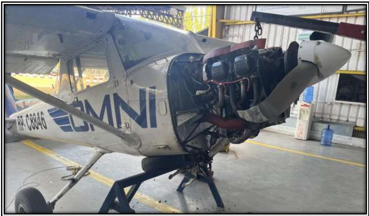
Figure 2. The aircraft damage nose landing gear and bent propeller blades
