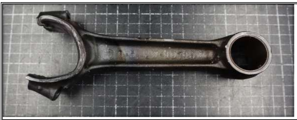
Figure 44 - The number 3 connecting rod in the as-received condition. The connecting rod experienced significant contact and heat damage. The connecting rod cap, bolts, nuts, and bearings were all separated from the assembly.
