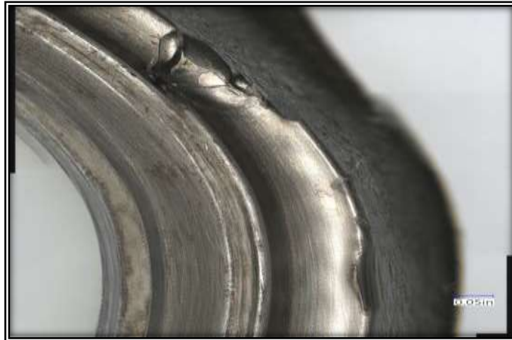
Figure 55 - The contact damage sustained to the outer circumference of the number 1 connecting rod.
