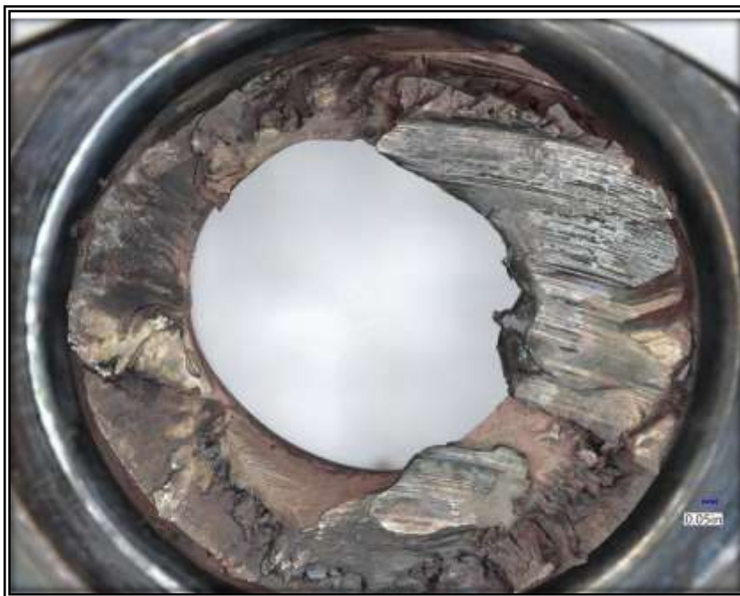
Figure 22 - 20x original magnification stitched image of the fracture surface from the rear sample.
