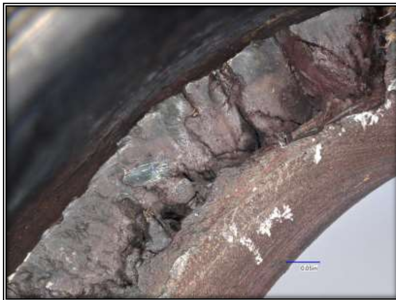
Figure 17- Subsurface cracking is present in a region of overload failure.
