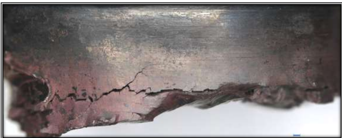
Figure 25. Original magnification of the side view of the top fracture surface from the rear sample, rotated 90 degrees clockwise.
