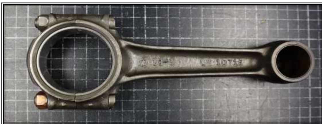
Figure 53 - The number 1 connecting rod in the as-received condition. Minor signs of wear and damage were observed.
