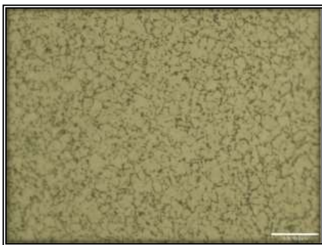
Figure 34 - 500x original magnification of the case microstructure of the sectioned rear sample after being etched with nital.
