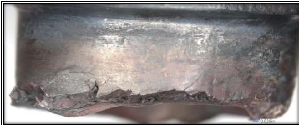
Figure 20 - 30x original magnification of the side view of the fracture surface from the front sample.
