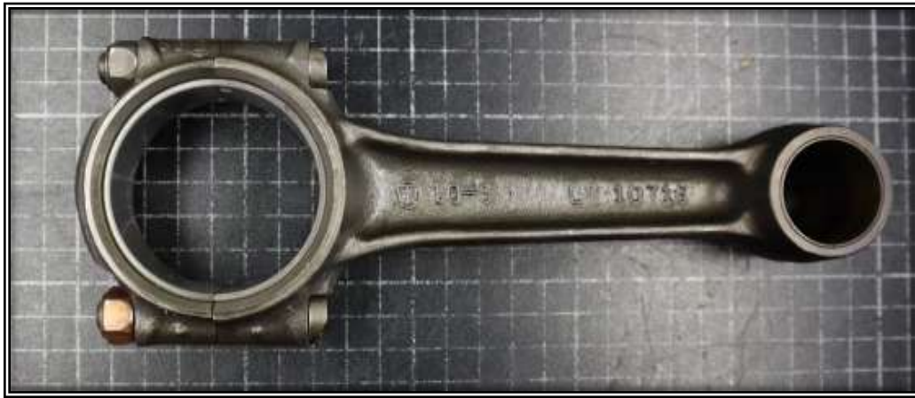
Figure 57 - The number 2 connecting rod in the as-received condition. Minor signs of wear and damage were observed.
