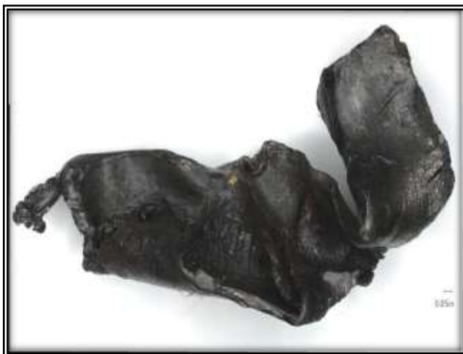
Figure 50 - Additional damaged pieces returned along with the number 3 connecting rod. The two pieces appears to be the damaged bearings associated with this connecting rod assembly. Both bearings have sustained significant material loss, deformation, and heat discoloration.
