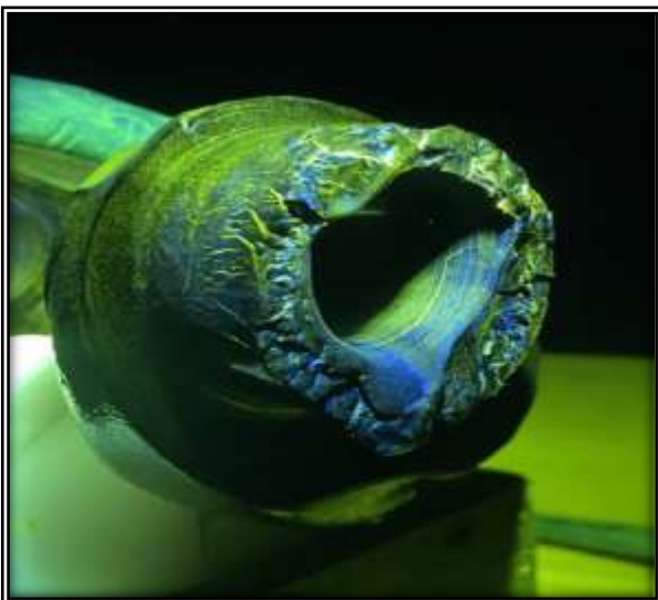
Figures 14 and 15 - Front sample surface during fluorescent dye mag particle inspection
