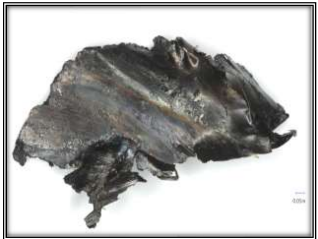
Figure 50 - Additional damaged pieces returned along with the number 3 connecting rod. The two pieces appears to be the damaged bearings associated with this connecting rod assembly. Both bearings have sustained significant material loss, deformation, and heat discoloration.
