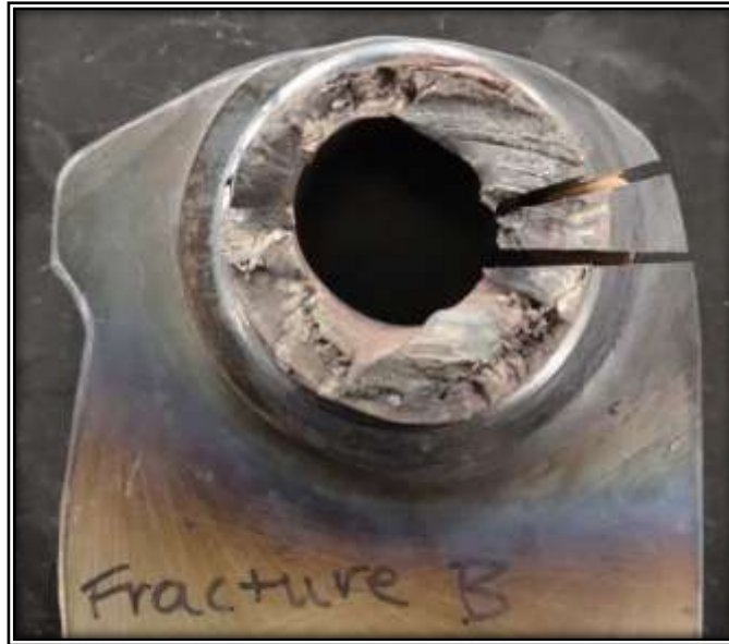
Figure 29. Reference location for the sectioned sample obtained from the fracture surface of the rear sample.
