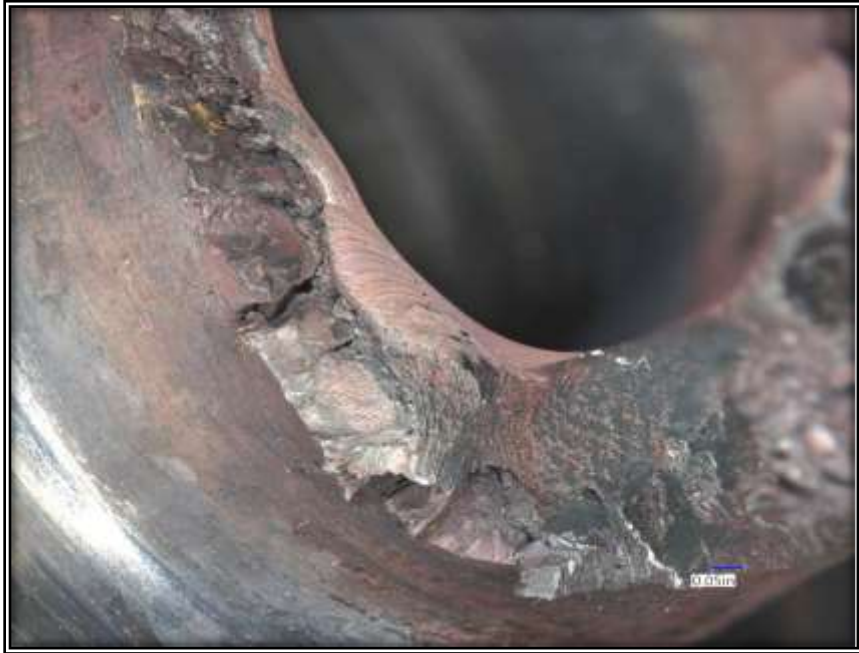
Figure 18 - 20x original magnification of the smeared metal on the fractured surface.
