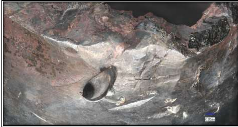
Figure 21 - 20x magnification of the damage on the outer diameter of the number 3 Pin on the front sample.
