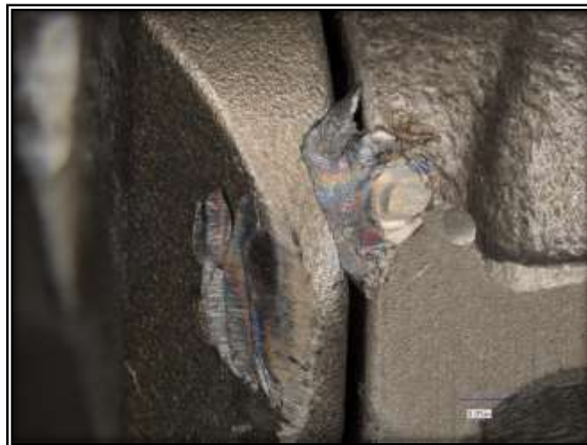
Figure 61 - Damage sustained to the number 4 connecting rod in the region of the connecting rod bolt. Material is smeared from contact damage and displays signs of heat tinting.
