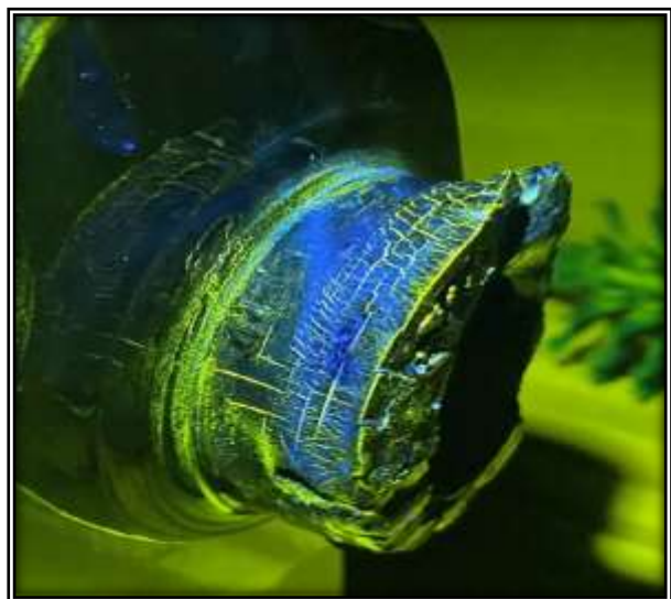
Figures 14 and 15 - Front sample surface during fluorescent dye mag particle inspection
