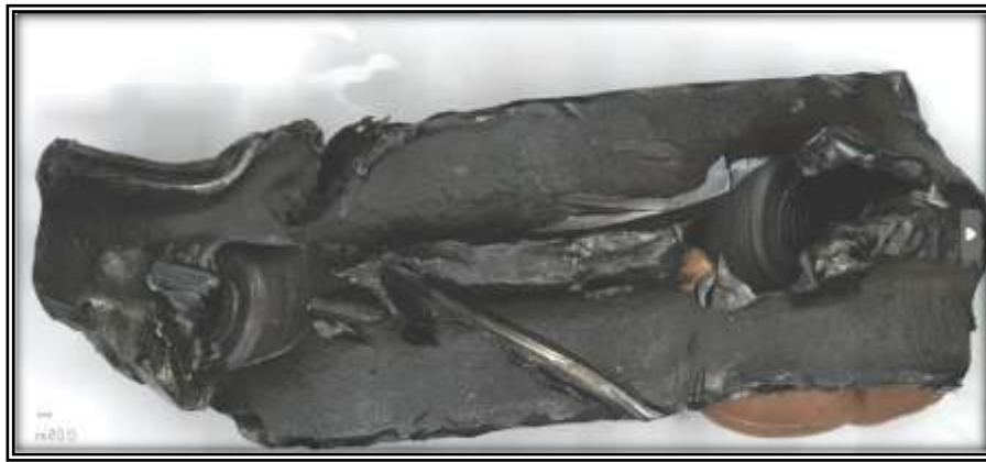
Figure 49 - The number 3 connecting rod cap piece. Significant deformation occurred to the shape of the cap, along with deep gouging on the part surface.
