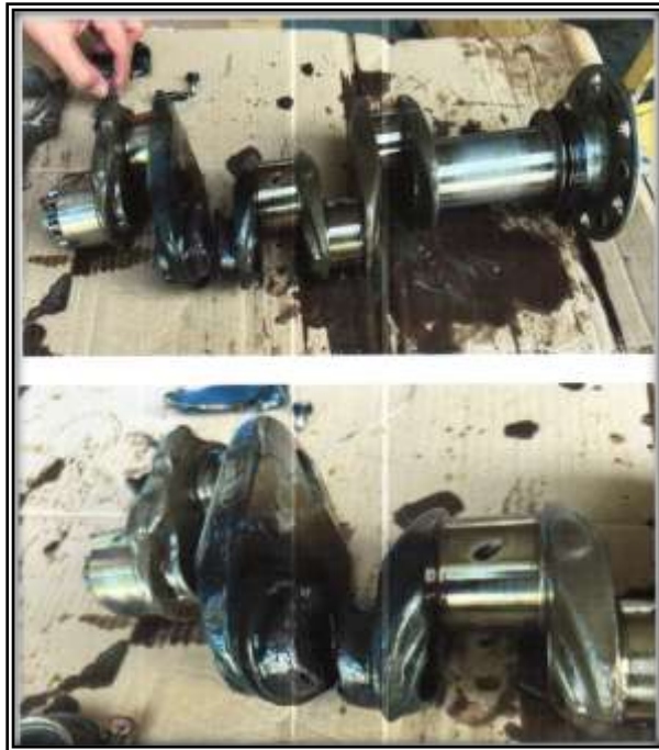
Figure 6 - Crankshaft assembly fractured at crank pin journal number 3.
