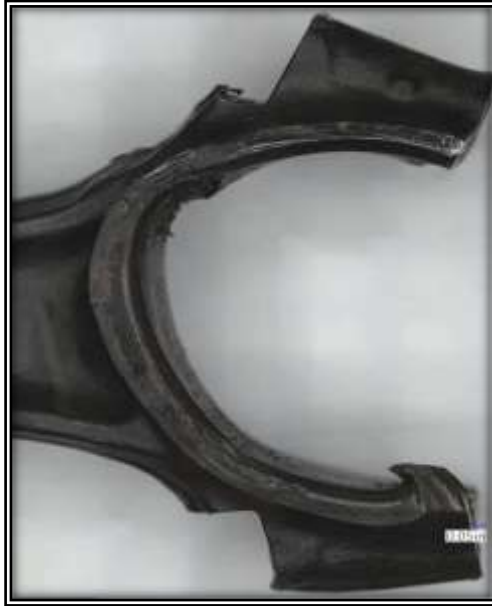
Figure 47 - Additional damage sustained to the number 3 connecting rod. The connecting rod is bent out of round with material cracking along the contact surfaces.
