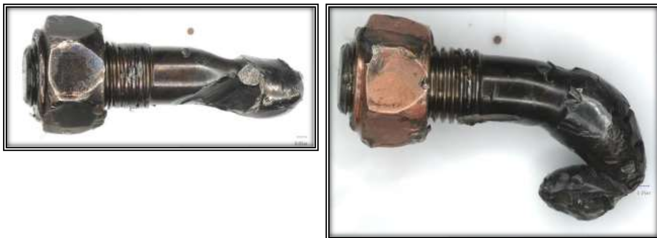
Figure 52 - Two remaining halves of the fractured connecting rod bolts along with their associated nut. Both bolts are fractured in the stem and contain significant deformation and gouging.
