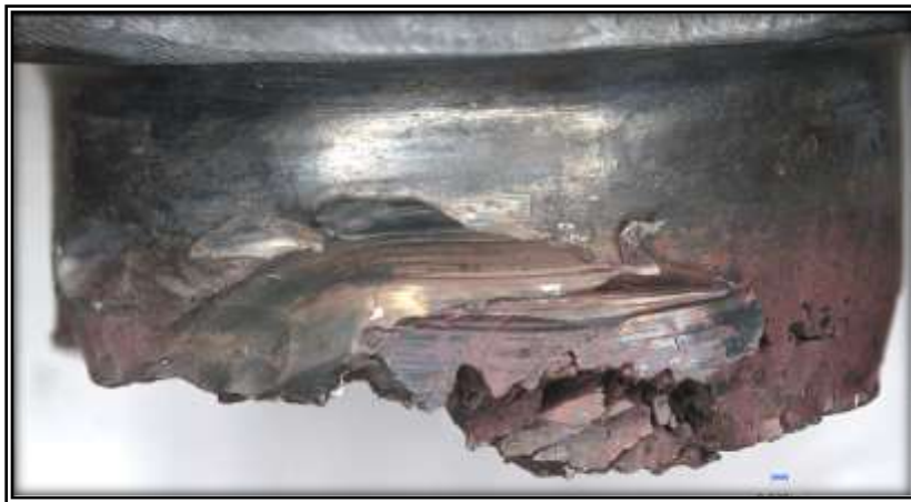
Figure 24 - 30x original magnification of the side view of the top fracture surface from the rear sample.
