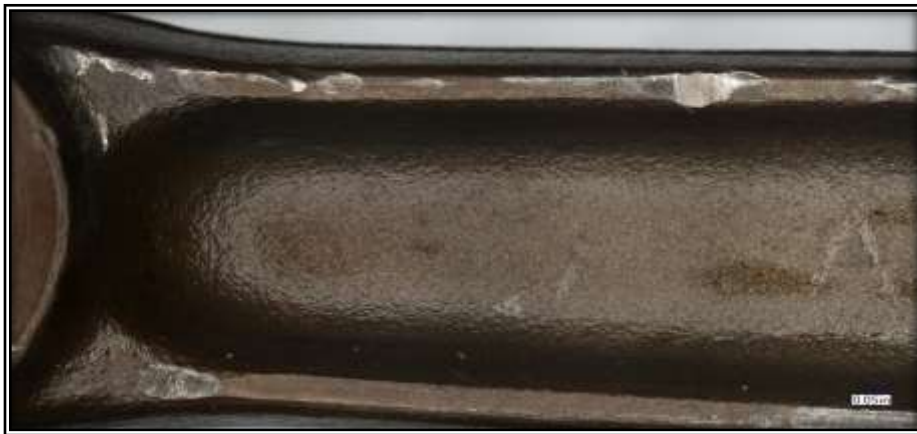
Figure 60 - Damage sustained to the I-beam section of the number 4 connecting rod
