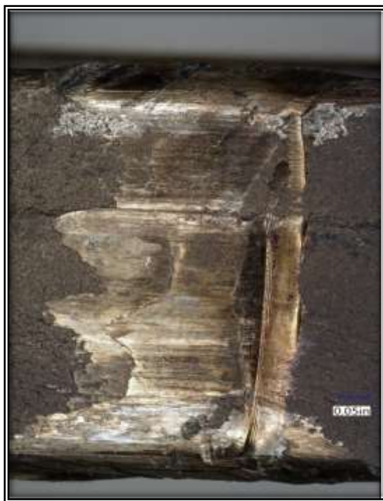
Figure 46 - Additional damage sustained to the number 3 connecting rod, noted by the deep gouge and material smearing.
