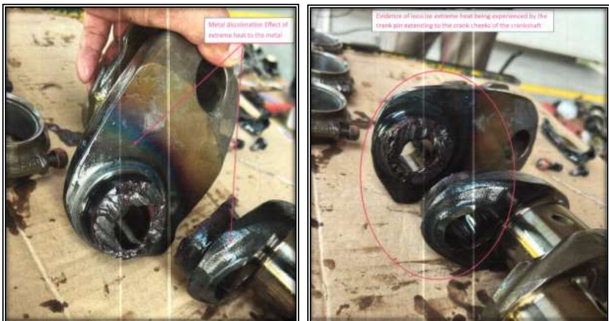
Figures 7 and 8 - The metal discoloration due to extreme heat.
