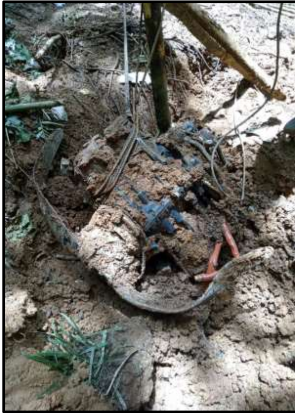
Figure 4 - The aircraft engine with its propeller buried in the ground.
