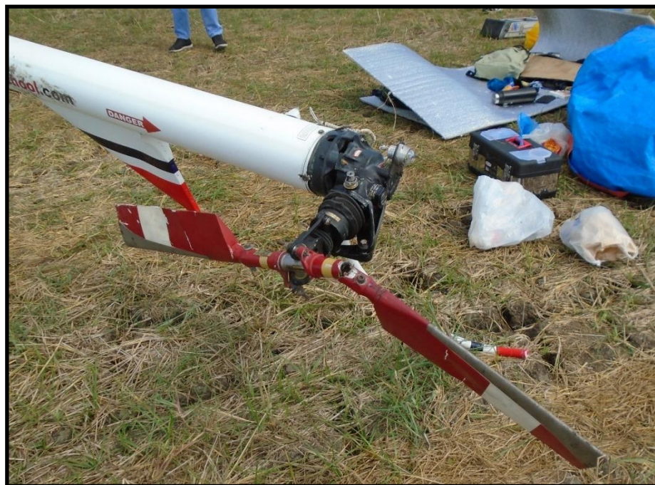
Figure 3 – Damaged tail rotor
