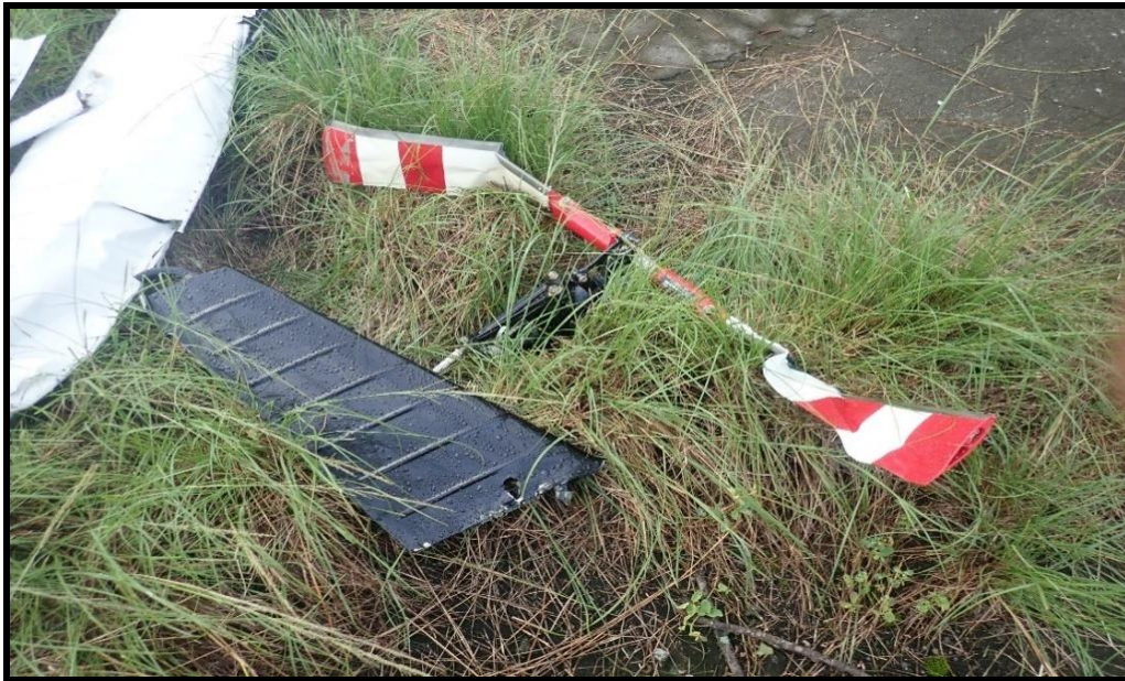
Figure 9. The detached Tail Rotor and other tail components at initial impact point.
