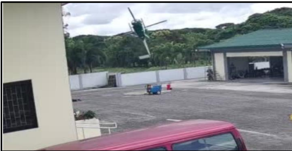
Figure 7. Helicopter tail impacts the ground first.
