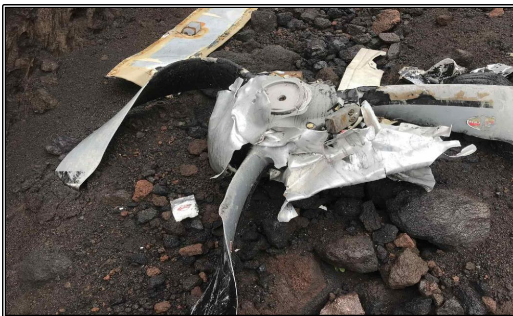
Figure 4 – The left propeller.
