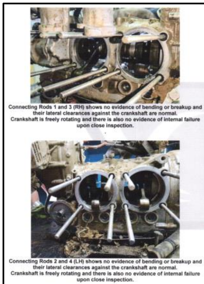
Figure 5 – Engine connecting rods during the top overhaul inspection
