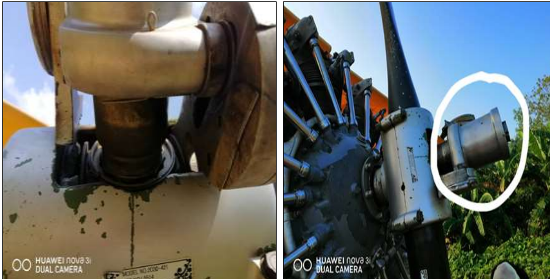
Figure 6 - Showing the broken counterweight bracket.
