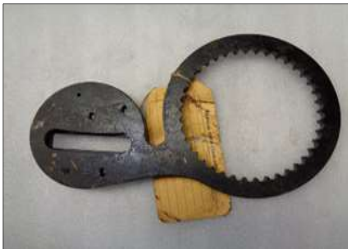
Figure 8 - A Propeller Counterweight Bracket.
