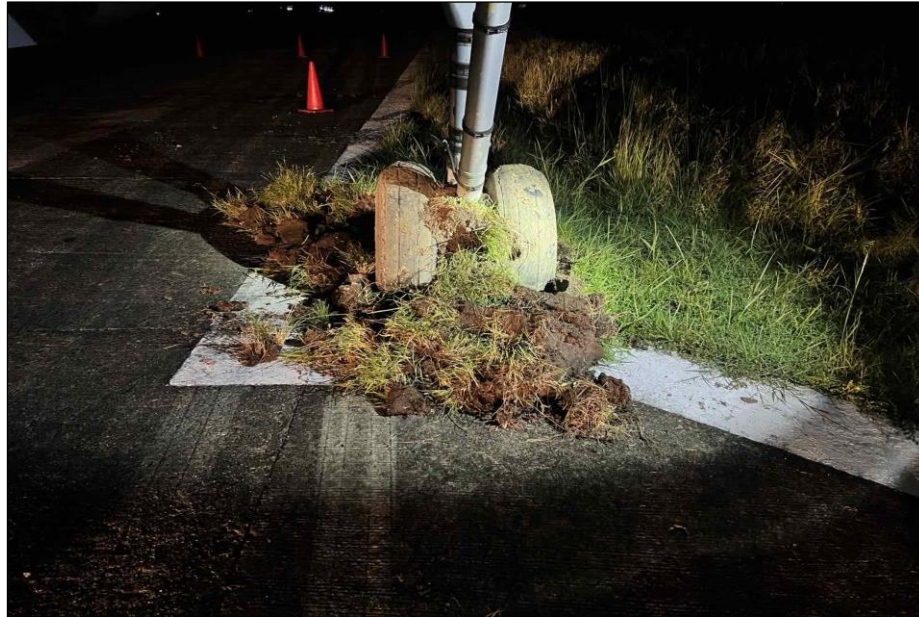
Figure 2 - The left main landing gear lodged on the soft ground.
