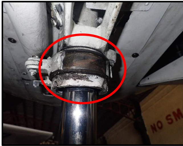
Figure 5 - Nose landing gear upper torque link assembly damage.
