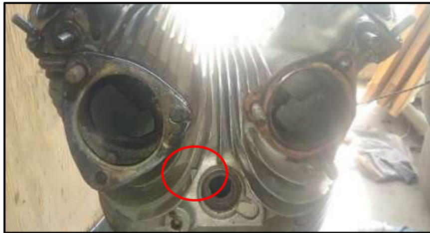
Figure 6: Visible crack where the oil was coming out.
