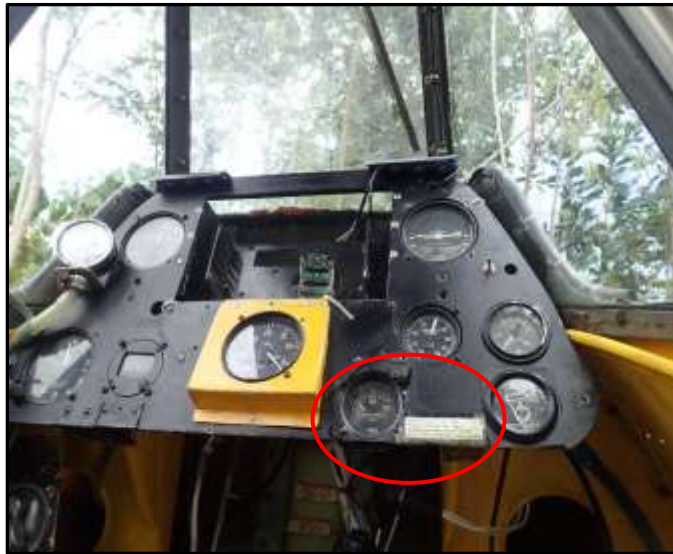
Figure 3 – RP-R5830 Cylinder Head Temperature (CHT) gauge with placard.
