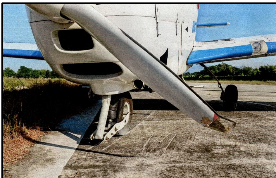
Figures 4 and 5 – The aircraft with its collapsed nose landing gear.
