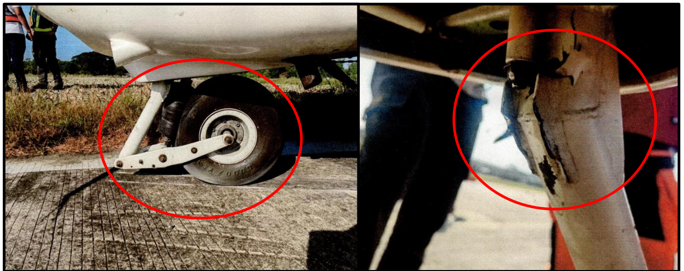
Figure 2 – Broken nose landing gear assembly.
