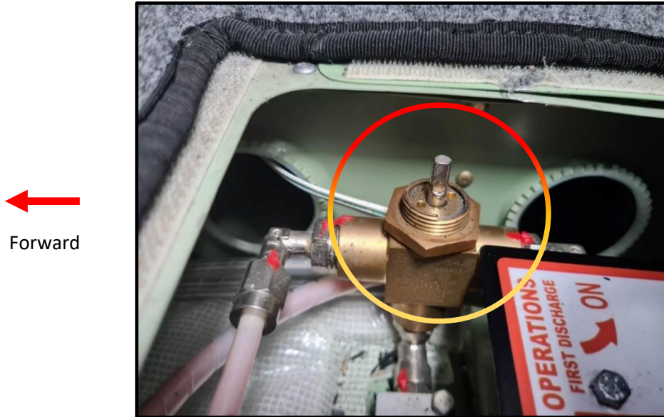
Figure 4 – The missing RH emergency landing gear valve lever.
