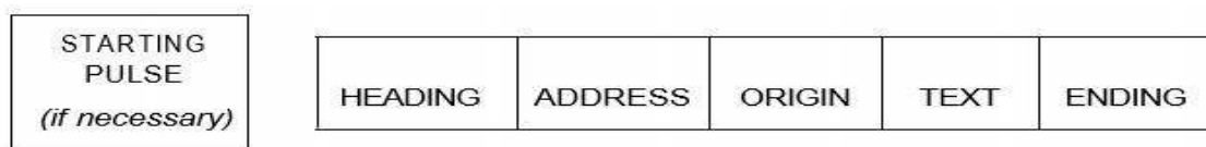
Figure 2.4-2. Form of transmission – teletypewriter operation (see 2.4.4.10.1.2)
