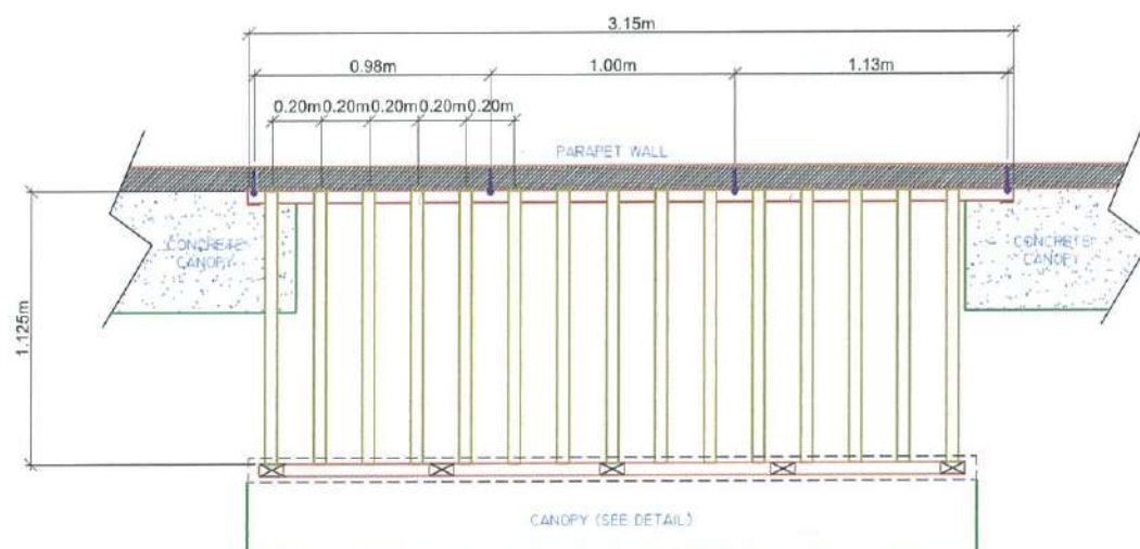
16 S-6 S-6 SCALE 1:20 mts DETAIL SECTION OF TRELLIS
