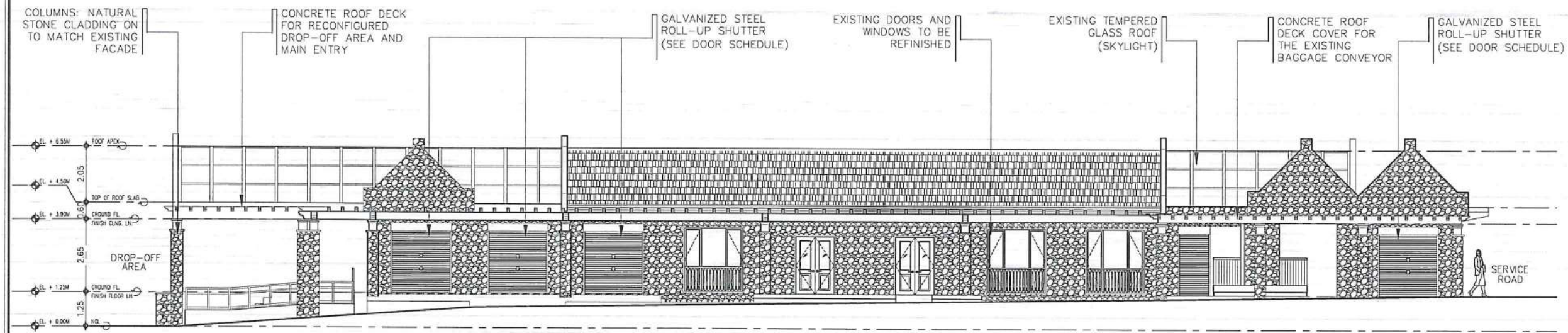
1 ELEVATION @ AIRSIDE SCALE: 1:175M
