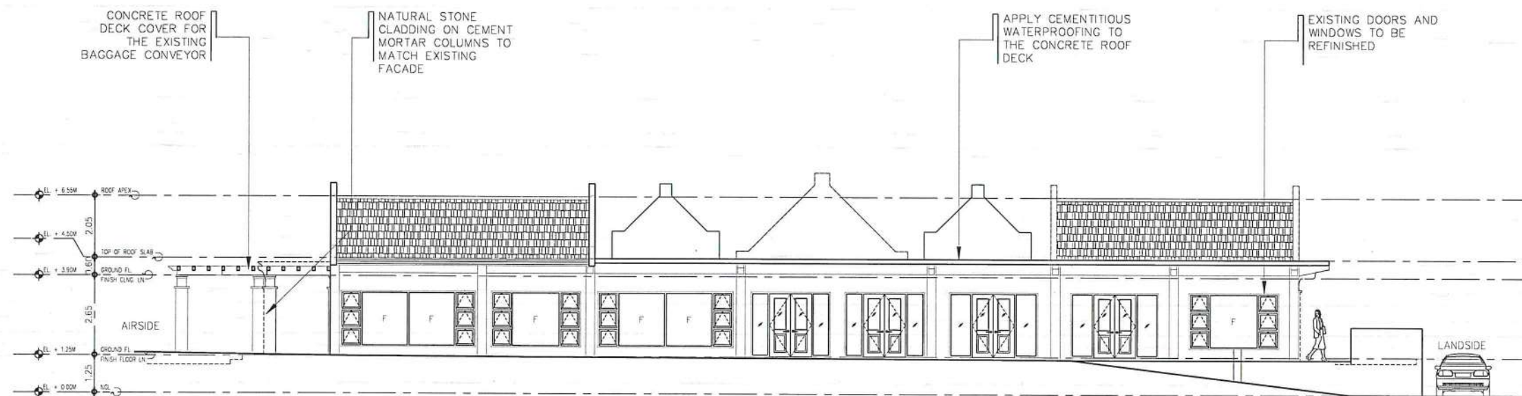
2 ELEVATION @ SERVICE ROAD SCALE: 1:175M
