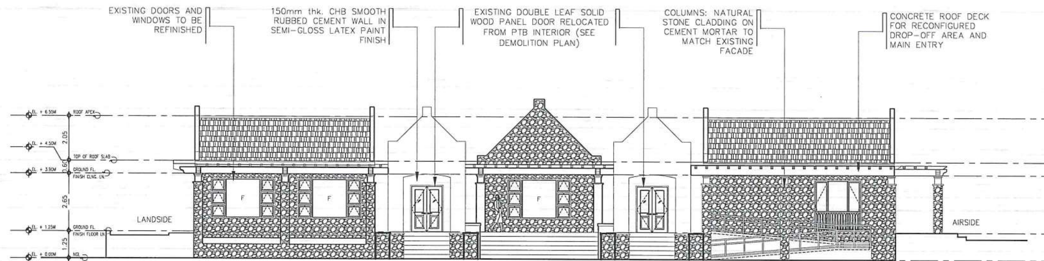
1 ELEVATION @ DROP-OFF SCALE: 1:175M
