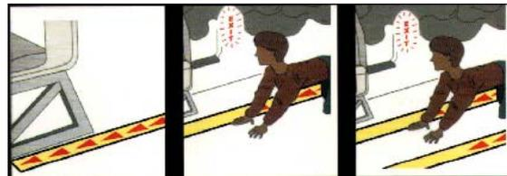
D. The PBC should depict the light colors indicating where the passenger is in respect to the emergency exit—
