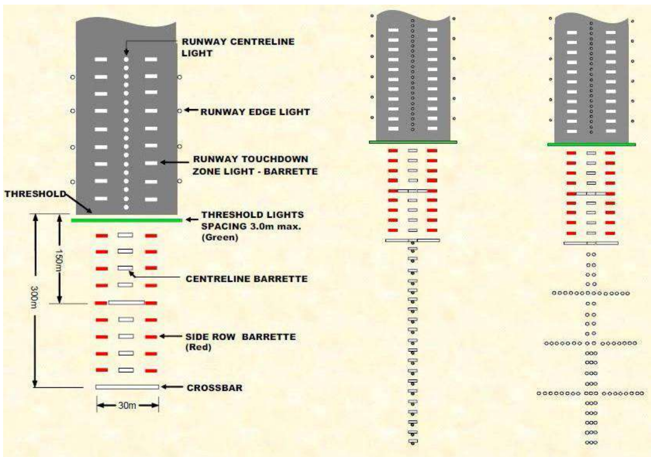
Figure 9.6-2: Illustration of category II and III approach lighting system
