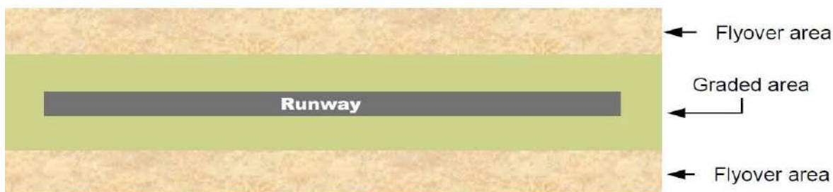
Runway strip consisting of both graded and fly-over area – instrument runways
