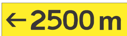
Figure 8.6-19: Take-off run distance available sign
