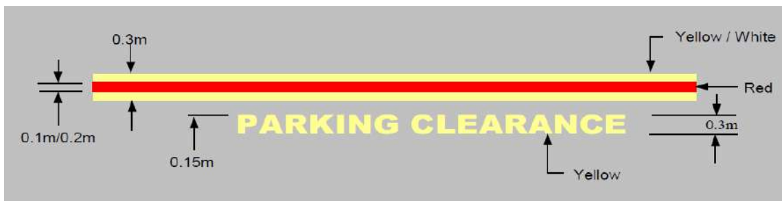
Figure 8.5-1: Parking clearance line
