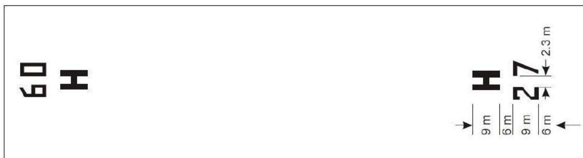
Figure 15-21. FATO designation marking and heliport identification marking for a runway-type FATO
