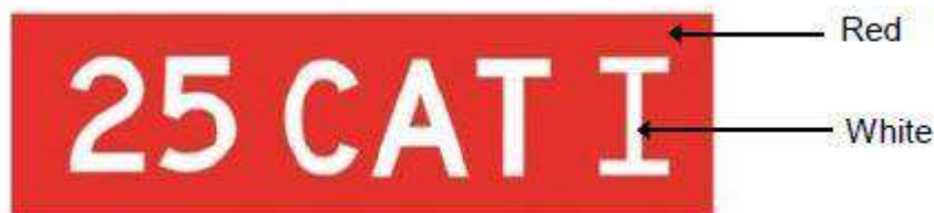
Figure 8.6-10: Category I runway-holding position sign
