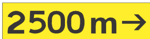
Figure 8.6-20 Take-off run distance available sign
