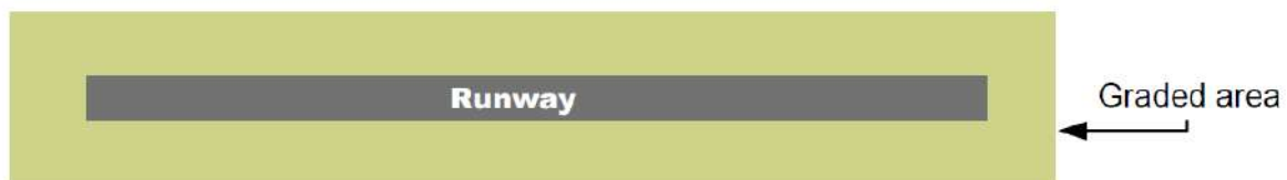
Runway strip consisting of fully graded area only – non-instrument runways
